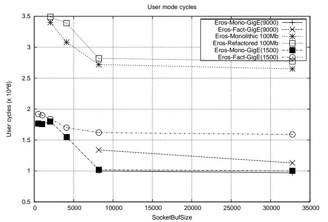
Figure 9: User cycles per 10,000 packets consumed during ttcp. Data for GigE(9000) for socketbuf lengths less than 8192 have been omitted to avoid graph compression. Measurements for smaller socket buffer sizes for the Gigabit (9000 mtu) case are limited by Linux transmit performance.
